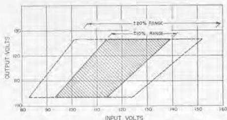
Figure 4. Range of operation for 115-volt models; for 230-volt models, multiply voltage scales by 2.
